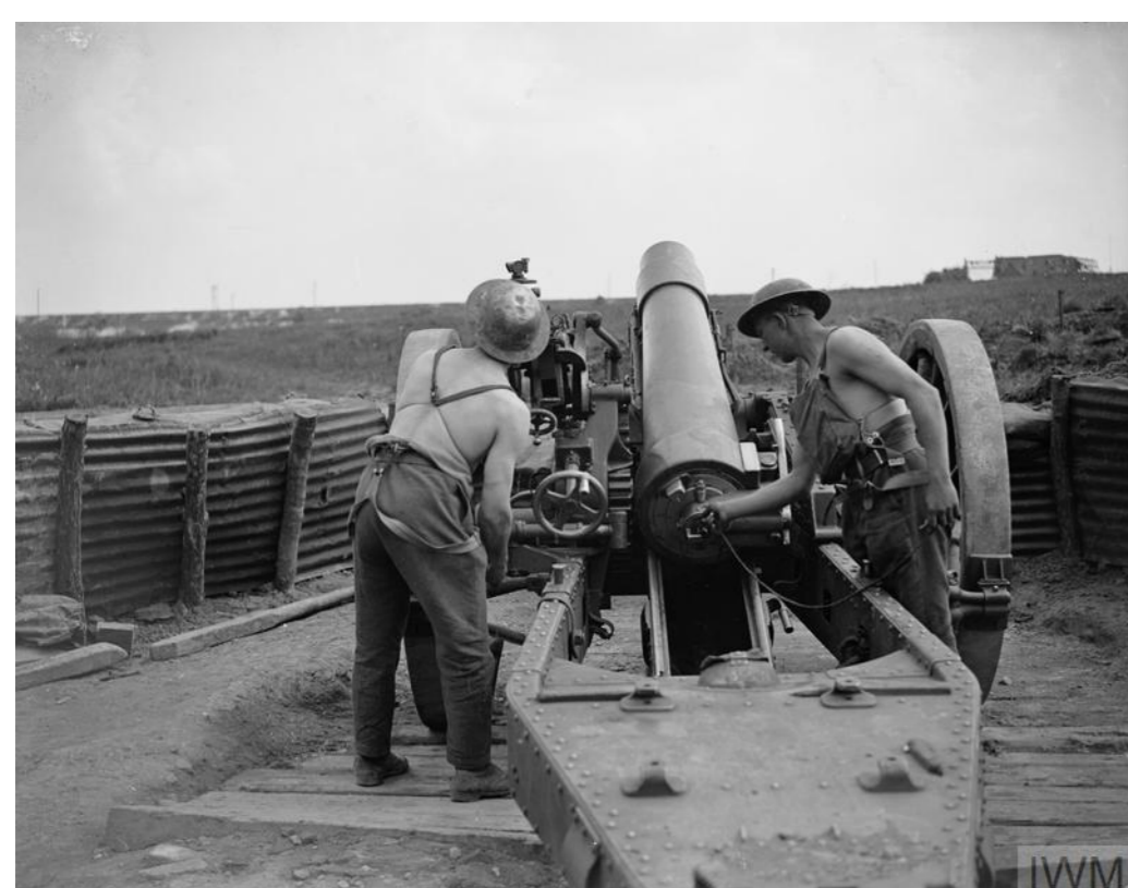
Crew of the 6-inch howitzer battery of the RGA sighting the howitzer and attaching the firing lanyard. 27 May 1918. IWM Q11029
